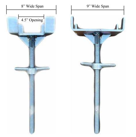
U-Head Screw Jack Dimensions: 9" x 8" U-Head Plate 4.5" Opening on 8" side of U-Head 24" Overall Height, 18" Adjustable Reinforced plates to increase load capacities
